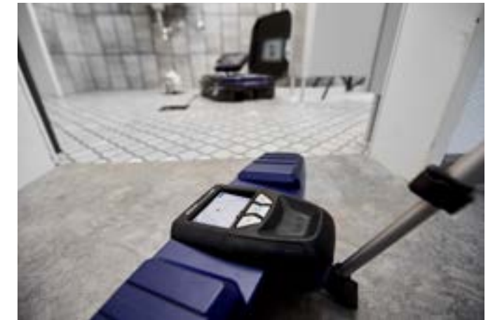
Precise location of the camera head with the Wöhler L 200 Locator, now with 512 kHz frequency
