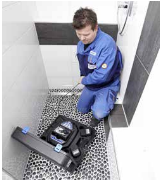
Wohler's new camera system is both compact and safely stored in a plastic case for transport and mobility.
