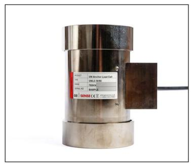
The Geosense® VWLC 5050 series of Vibrating Wire Load Cells consist of a solid cylinder of high strength steel with 3 or 5 vibrating wire strain sensors mounted parallel to the longitudinal axis arranged equidistant around the circumference which measure the compression of the cylinder under load.
