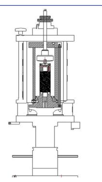
Fig 4.Schematic of double cell within a GDS Bishop and Wesley triaxial cell
