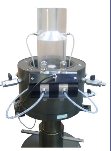
Fig. 3 Show HKUST inner cell with DPT attached to the front of the frame.
