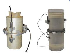
Fig. 6 Hall Effect and LVDT transducer
