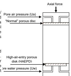
Fig. 1 Schematic of test specimen connections when using GDS Method A
