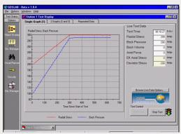
Fig. 9 Test display showing a 4D unsaturated stress path test in progress
