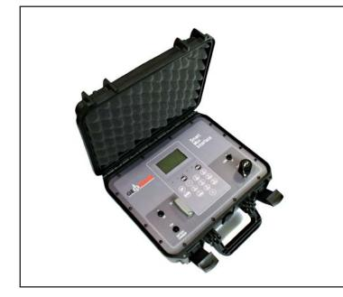
Sensor channels can be easily viewed and selected via the SmartMux Interface which replaces time-consuming rotary switches and readout.
