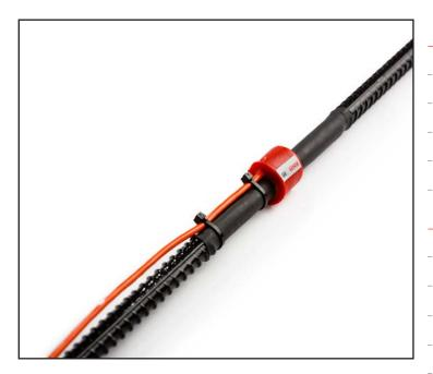
Geosense® VWS-4000 series vibrating wire Sister Bars and Rebar Strain Meters are designed to be embedded in concrete to measure strains due to imposed loads.
