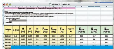
Olson's RTG software automatically exports results to our Calculations Spreadsheet that determines Young's Modulus, Shear Modulus and Poisson's ratio.
