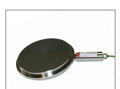
This consists of a sensitive pressure pad formed by joining two stiff steel discs at their periphery. The void inside the cell is filled with de-aired fluid. When load is applied to the cell the pressure of the inside liquid changes. The changes in pressure correspond directly to the load applied.
