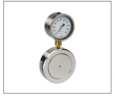
The Geosense® HLC-6050 series of Hydraulic Load Cells consist of a sensitive pressure pad formed by joining two stiff steel discs at their periphery. The void inside the cell is filled with de-aired fluid. When load is applied to the cell the pressure of the inside liquid changes. The changes in pressure correspond directly to the load applied.
