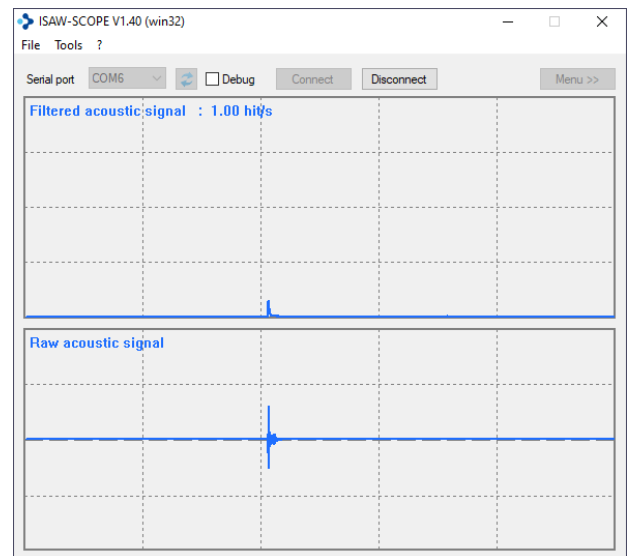
Field checking result in scope mode. This signature is similar to the response of the sensor to the impact of a 1.5 to 2.0 cm diameter hailstone at terminal velocity.
