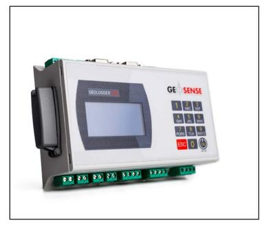
The Geosense GeoLogger G8 is a versatile low power multichannel data logger module which is capable of being used with a wide range of sensors with outputs which include VW, V, mV/V, 4-20mA, Pt100, NTC.
