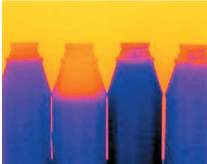
Detecting liquid levels in visually opaque bottles.
