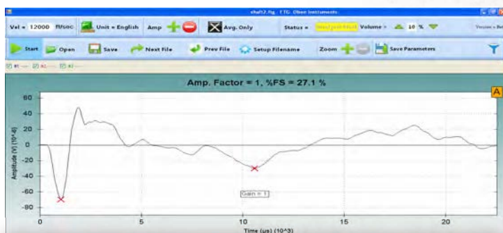
Olson's FTG Software showing sonic echo waveform
