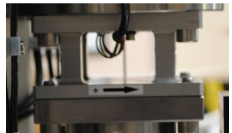
Fig. 6 Shear load cell located directly above sample
