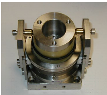
Fig. 8 Specimen top cap held above sample
