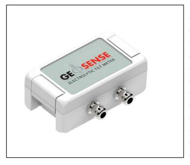
The Geosense® Digital EL In-Place Tilt Meter measures uniaxial or biaxial tilt, which is measured from the plane(s) perpendicular to the base.
