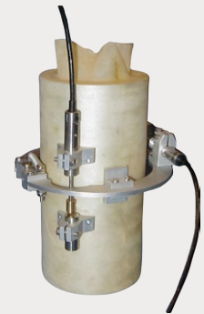
Fig 2. LVDT transducers as shown on sample.
