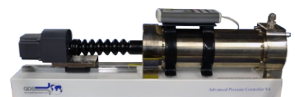
Fig 3. Advanced Pressure Controller used in Unsaturated Testing
