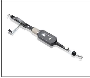
The Digital Tape Extensometer is a portable device used for measuring displacement between reference anchors fixed to an excavation or structure.
