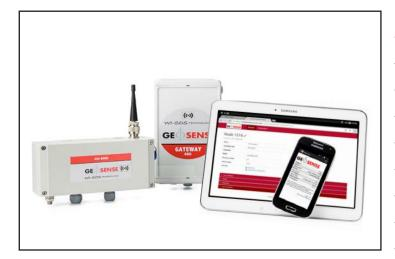
The Wi-SOS 480 (Wireless Sensor Observation System) provides a system to transmit, receive and data log remotely signals from any sensor with a vibrating wire, voltage, 4-20mA, SDI12 or resistance output over long ranges up to 15 km.
