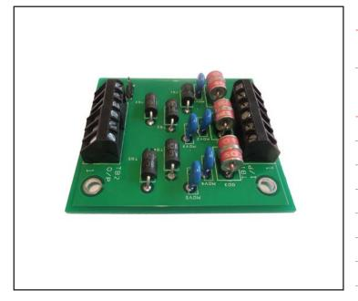
Geosense® Surge Protective Device (SPD) protects all types of sensors from transient overvoltage.
