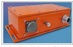
The KMPS-3-64 is a 64 position pressure scanner with high accuracy digital output over either an RS-485 or Ethernet bus. There is an internal heater which keeps the internal temperature above freezing to avoid internal icing. An optional motor allows for digital control over the purge mechanism. The KMPS also features auto-zero capabilities. The KMPS-3-64 has a water resistant case ideal for outdoor testing.
