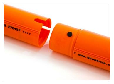
Geosense<sup>®</sup> QJ Inclinometer Casing is a quick connecting casing, precision extruded from ABS, with four precise keyways formed at 90 degrees which allow accurate installation of portable and in-place inclinometers.
