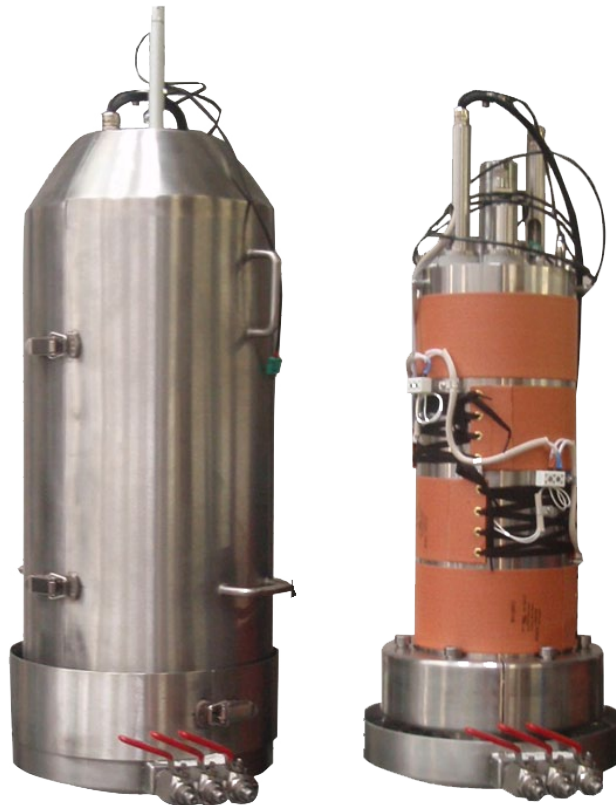
20MPa high pressure cell with the temperature control.
