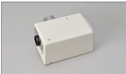
Motorized DSC zooming port (Ni-E) A digital camera can be mounted on the camera port. A motorized 0.6X - 2.0X zoom optical system is incorporated.
