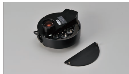
Motorized excitation filter wheel (Ni-E) Excitation filter positions (8 positions—using 25mm filters) can be changed at a high speed of 0.15 sec. between adjacent positions.
