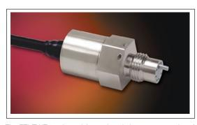
The ETL/T-HT-375 is a miniature threaded pressure transducer/ platinum RTD combination. The pressure transducer utilizes a patented silicon on silicon design. The platinum RTD protrudes beside the diaphragm to sense media temperature. The pressure and temperature devices are designed to operate independently. All wetted parts of the transducer are compatible with most industrial and automotive fluids.
