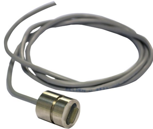
Fig 3. GDS Titanium Bender Element Insert
