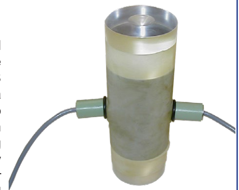
Fig 2. Horizontal elements mounted to specimen
